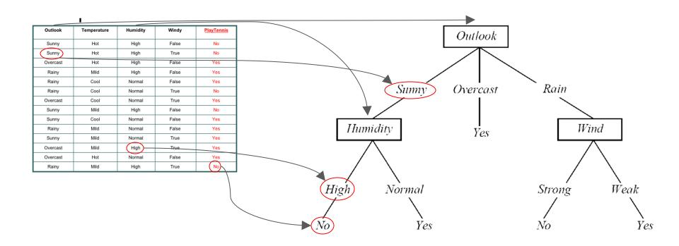
→ A DT uses the <u>features</u> of an observation table as nodes and the <u>feature values</u> as links.
